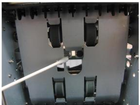
GUIDE OPEN→ Clean by using of cotton swab the optical sensor and surface and reflected lens of sensor.
