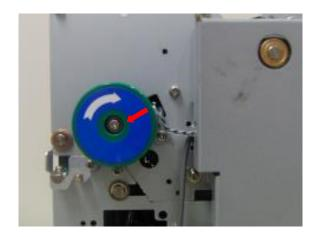
② Loosen and remove one screw on the sensor bracket according to the picture.
