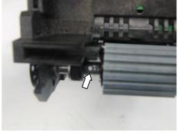
② Loosen and remove two screws, pull two hinge pins off the cassette.
