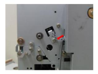
③ Pull sensor bracket out of the frame according to the picture.
