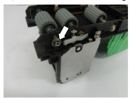
② Loosen and remove two screws on the other side of wheel lock, and remove the bracket & bearing
